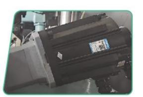
The station mold closing, forming auxiliary stretching, and pull-tab parts are all driven by servo motors, which have fast speed, low noise, high precision, and high efficiency.
